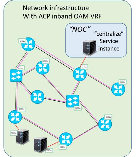
ACP secure virtual connections With GRASP signaling ACP: Autonomic Control Plane
