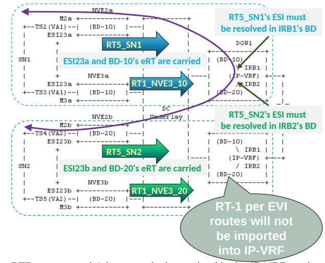
Notes1: These RT5 routes needn't be recursively resolved in the IP-VRF routing • RT-1 per EVI routes are importable, because that its L3 out interface (the IRB interface of BD-10/BD-20) can be directly determined by the route-targets carried in itself.
