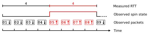
The **sQuare bit** creates square waves of a known length as defined in the Alternate Marking (RFC8321). This can be used for packet loss measurements.
