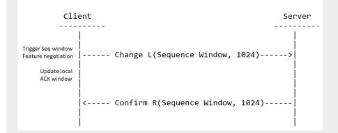
New or enhanced feature for Sequence Window negotiation in DCCP required?
