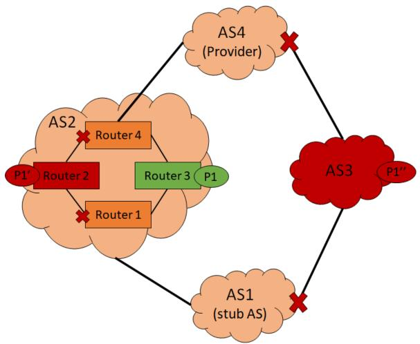
P1 is the source address prefix of Router3 P1' is the spoofed P1 by Router2 P1'' is the spoofed P1 by routers in AS3  Intra-AS SAV avoids source address spoofing from inner AS
