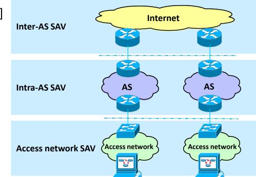
It is difficult to require all access networks to deploy SAVI simultaneously, so Intra-AS SAV and Inter-AS SAV are more encouraged by MANRS
