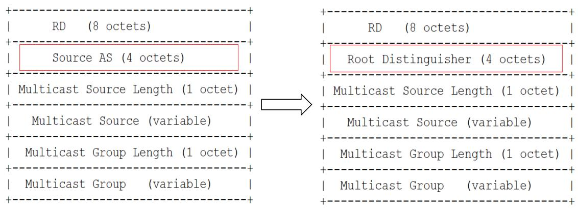
In IPv6 underlay networks, "Root Distinguisher" field is an root index locally assigned by the originator of the C-
