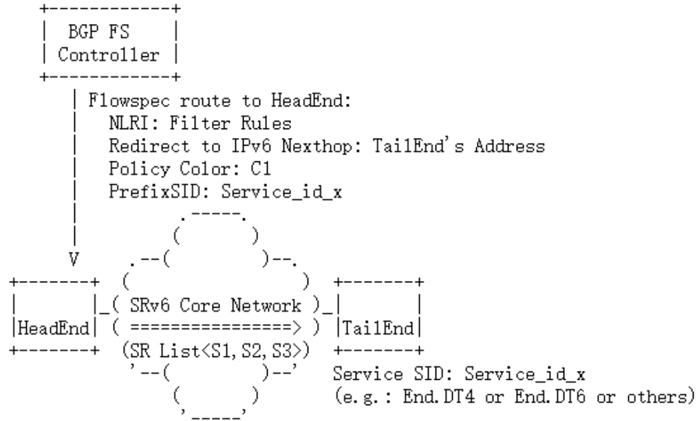
Figure 1: Steering the Flow into SRv6 Policy (Option 1)
