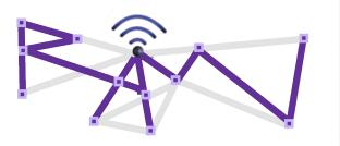
RAW OAM operation in the Network Plane observes either a full Track or subTracks that are being used at this time. In the case of Radio Access Protection, the Track is Loose and only the first hop is observed:
