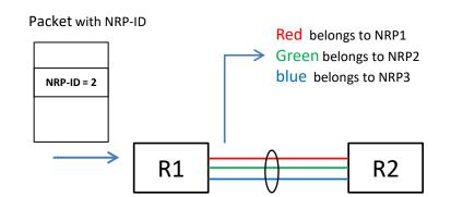
R1 gets NRP-ID from packet and Determines the Green line to forward packet
