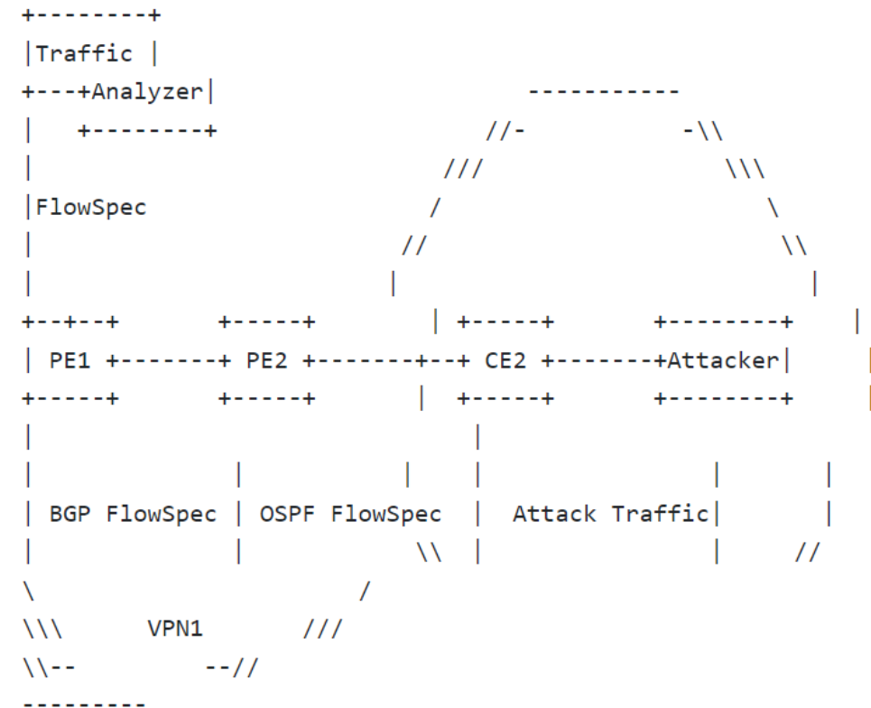
Figure 2: Traffic Analyzer deployed in Provider Network
