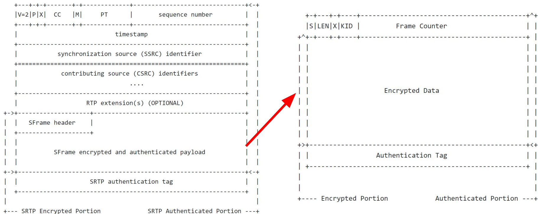
Figure 1: SRTP packet with SFrame-protected payload
