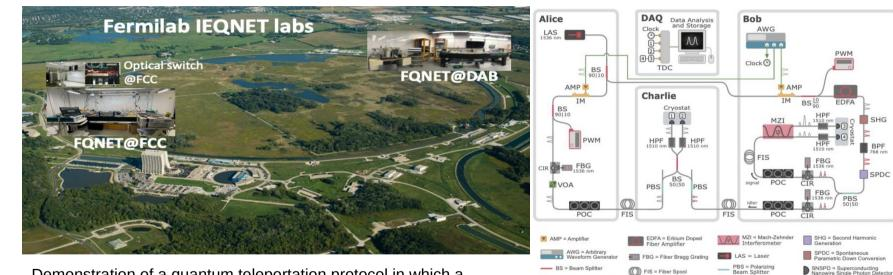
Demonstration of a guantum teleportation protocol in which a photonic qubit (provided by Alice) is interfered with one member of an entangled photon-pair (from Bob) and projected (by Charlie) onto a Bell-state, whereby the state of Alice's qubit can be transferred to the remaining member of Bob's entangled photon pair.
