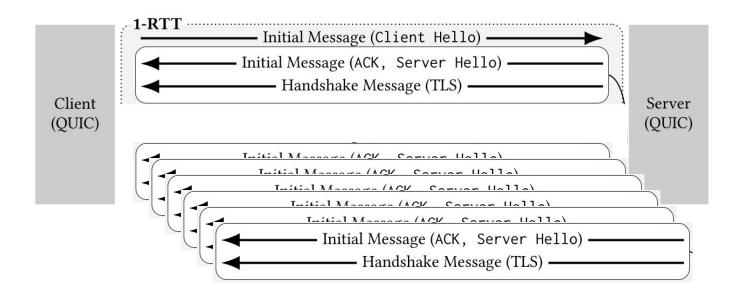
Servers that experience incomplete handshakes assume packet loss and resend packets, which can lead to high amplification factors.
