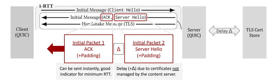
Pro: This keeps ProbeTimeouts for RTT estimation low. Con: But it leads to larger handshake data (>3x).
