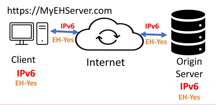
This works. We have managed to send EH to Origin Server by bypassing CDN Proxy. Now we are back to simple client / server scenario
