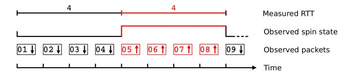
The sQuare bit creates square waves of a known length as defined in the Alternate Marking (<u>RFC 9341</u>). This can be used for packet loss (and delay) measurements.
