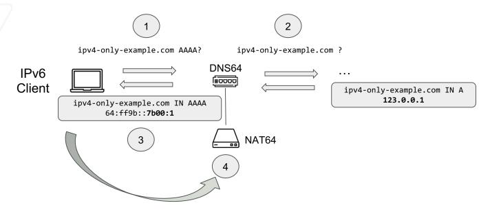
DNS64 maps IPv4 address to an IPv6 address
