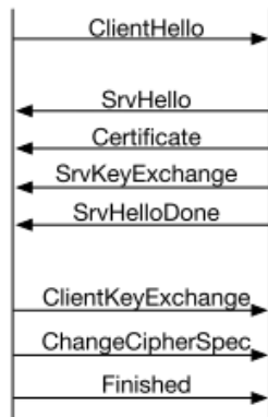
Figure 2: TLS 1.2 Handshake Messages.
