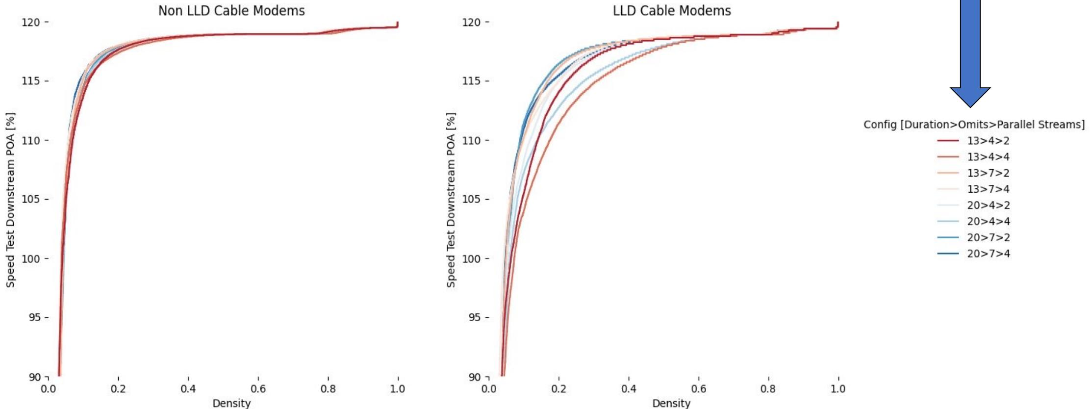
Speed test downstream performance as measured by percent-of-advertised (POA) speed achieved from non-errored tests ran on 300, 500, 800, 1000 Mbps advertised speed tiers. The scheduler ran tests on non LLD and LLD cable modems using pre-selected configurations on PPODs: CABAPP106, CABJPP102, FLNDPP107.
