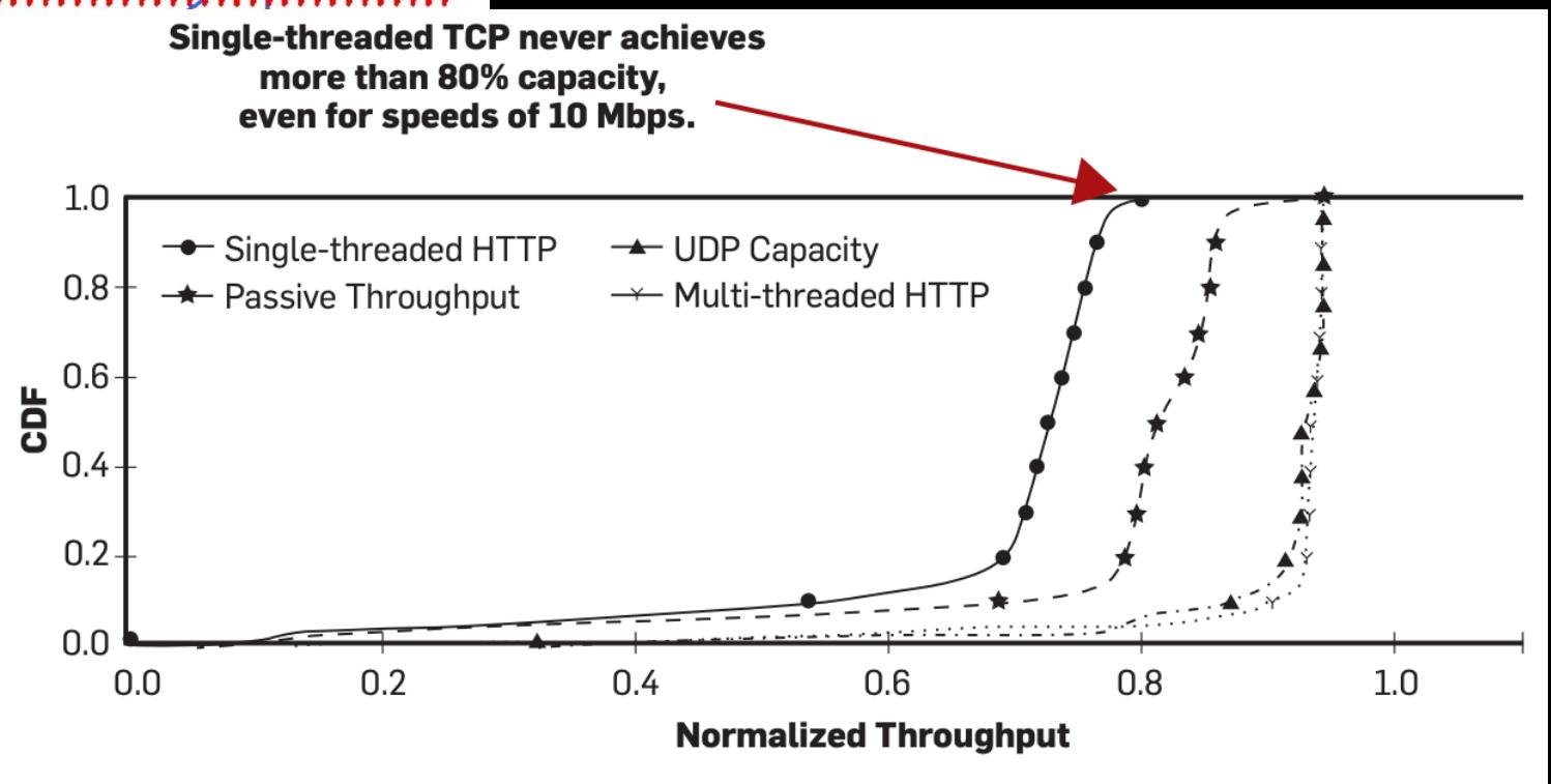
*One connection insufficient for aggregate capacity test, hence parallel connections*
