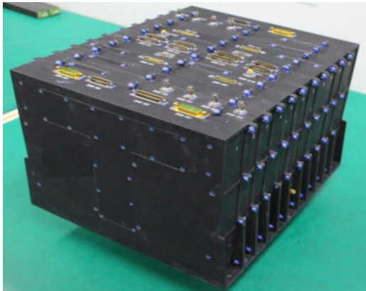
high-speed router for space network I
