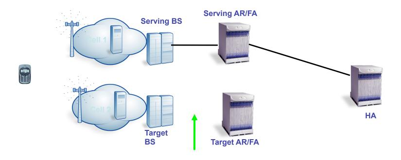
HA bi-cast can be a configurable feature in the HA based on operator's policy. It is also possible that the Serving AR establishes a transport connection with the Target AR instead of HA bi-casting
