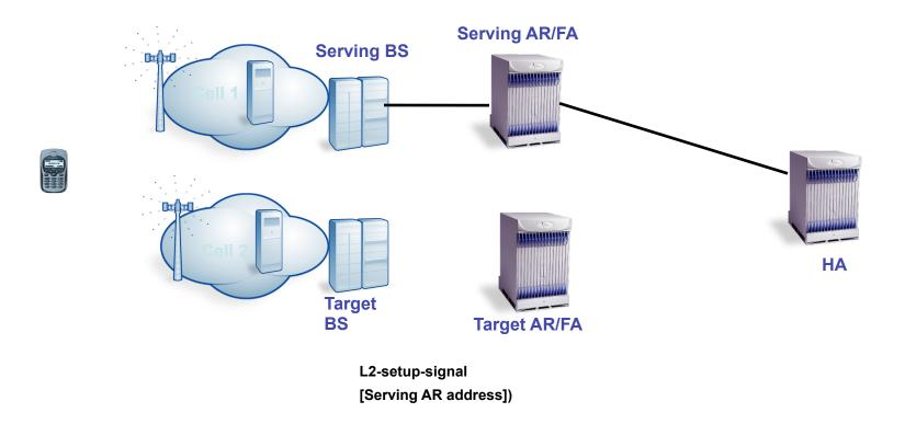
HA bi-cast can be a configurable feature in the HA based on operator's policy. It is also possible that the Serving AR establishes a transport connection with the Target AR instead of HA bi-casting
