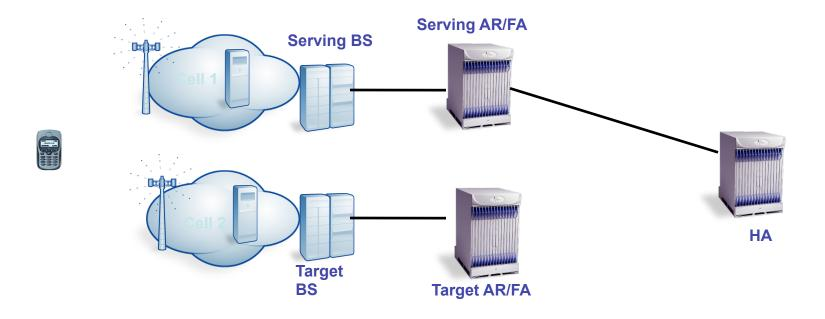
HA bi-cast can be a configurable feature in the HA based on operator's policy. It is also possible that the Serving AR establishes a transport connection with the Target AR instead of HA bi-casting
