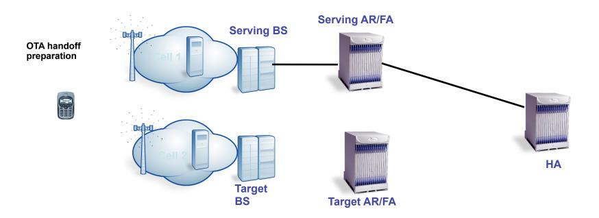
HA bi-cast can be a configurable feature in the HA based on operator's policy. It is also possible that the Serving AR establishes a transport connection with the Target AR instead of HA bi-casting
