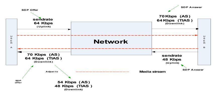
We need a bandwidth modifier in 'send' direction to signal the asymmetric bitrates of a bi-directional ('sendrecv') stream. This is also useful to signal the max bitrate of a 'sendonly' stream.
