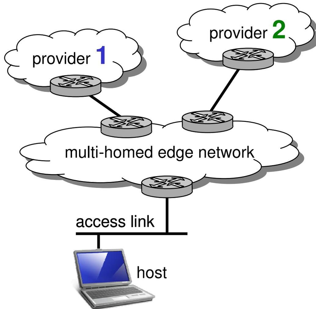
Edge network connects to multiple providers (increased bandwidth, provider services, fault-tolerance)
