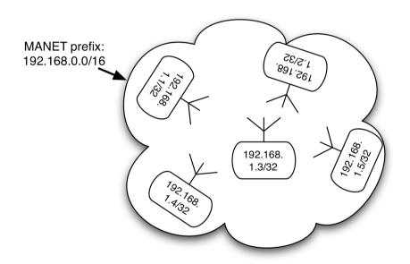
IP addresses assigned to MANET routers within the same MANET may be extracted from within a larger prefix, e.g. 192.168.0.0/16
