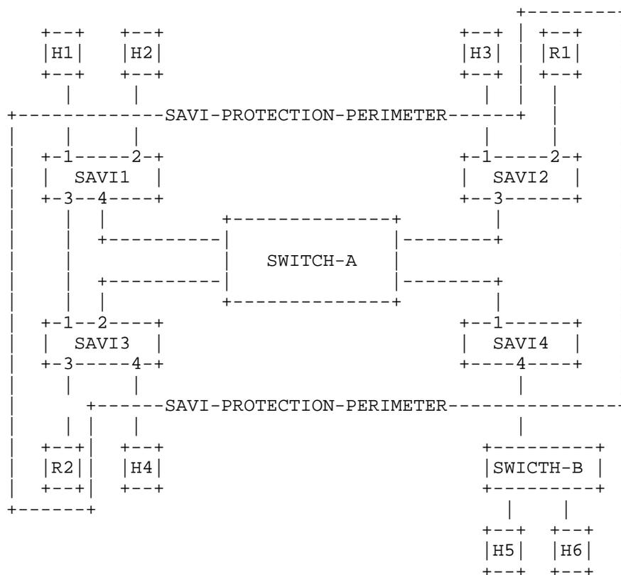
In the figure above, the FCFS SAVI protection perimeter is provided by 4 FCFS SAVI devices, namely SAVI1, SAVI2, SAVI3 and SAVI4. These devices verify the source address and filter packets accordingly.
