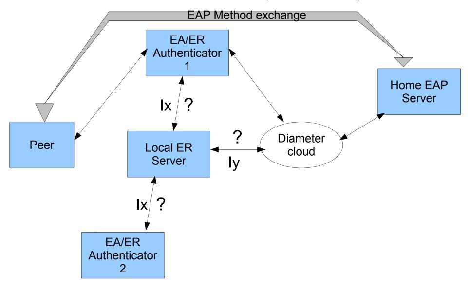
It seems very probable that **ly** is required, both for direct ER server to EAP server interaction for authorization and for consistency with RFC 5296 collocation case during authentication. **lx** is a possible alternative.
