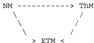
Figure 1: PCN Codepoint Re-Marking Diagram for Dual Marking (DM)
