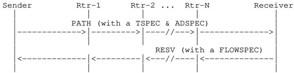
Figure 1. Concept of RSVP in a Single Direction
