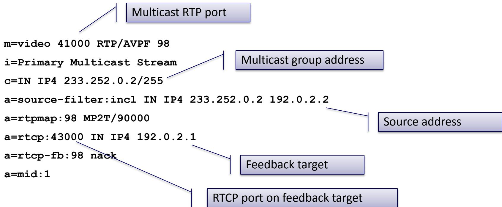
RTCP port associated with the SSM session cannot be specified by the 'rtcp' attribute. RFC 5760 says it must be derived from the "m=" line
