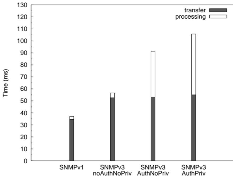
Figure: Time taken for transferring and processing an SNMP request.
