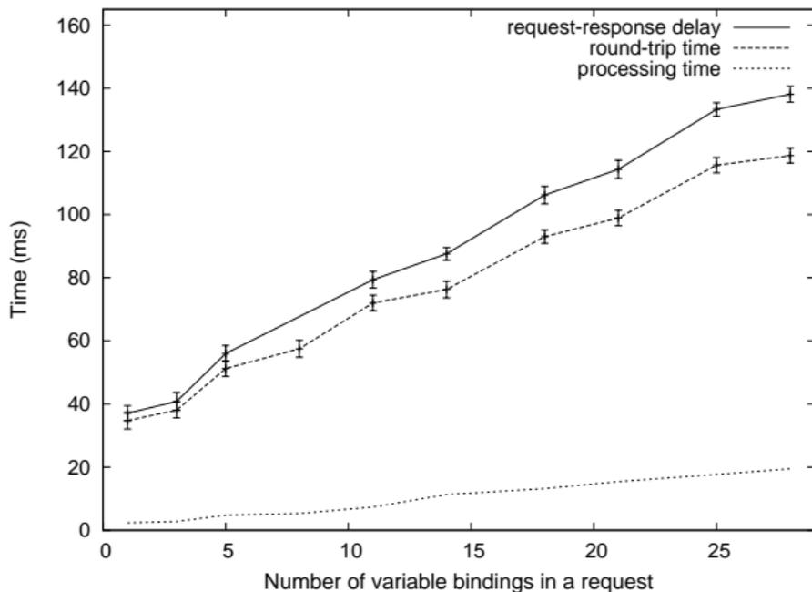
**Figure:** Time spent in transferring and processing SNMPv1 requests and responses as a function of the number of variable bindings in a request.
