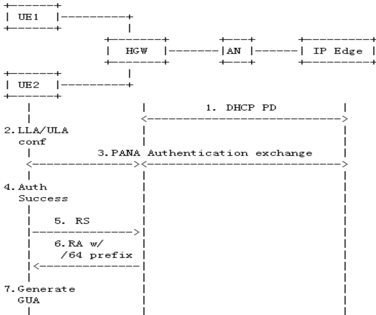
Figure 1: IPv6 Broadband Access Network
