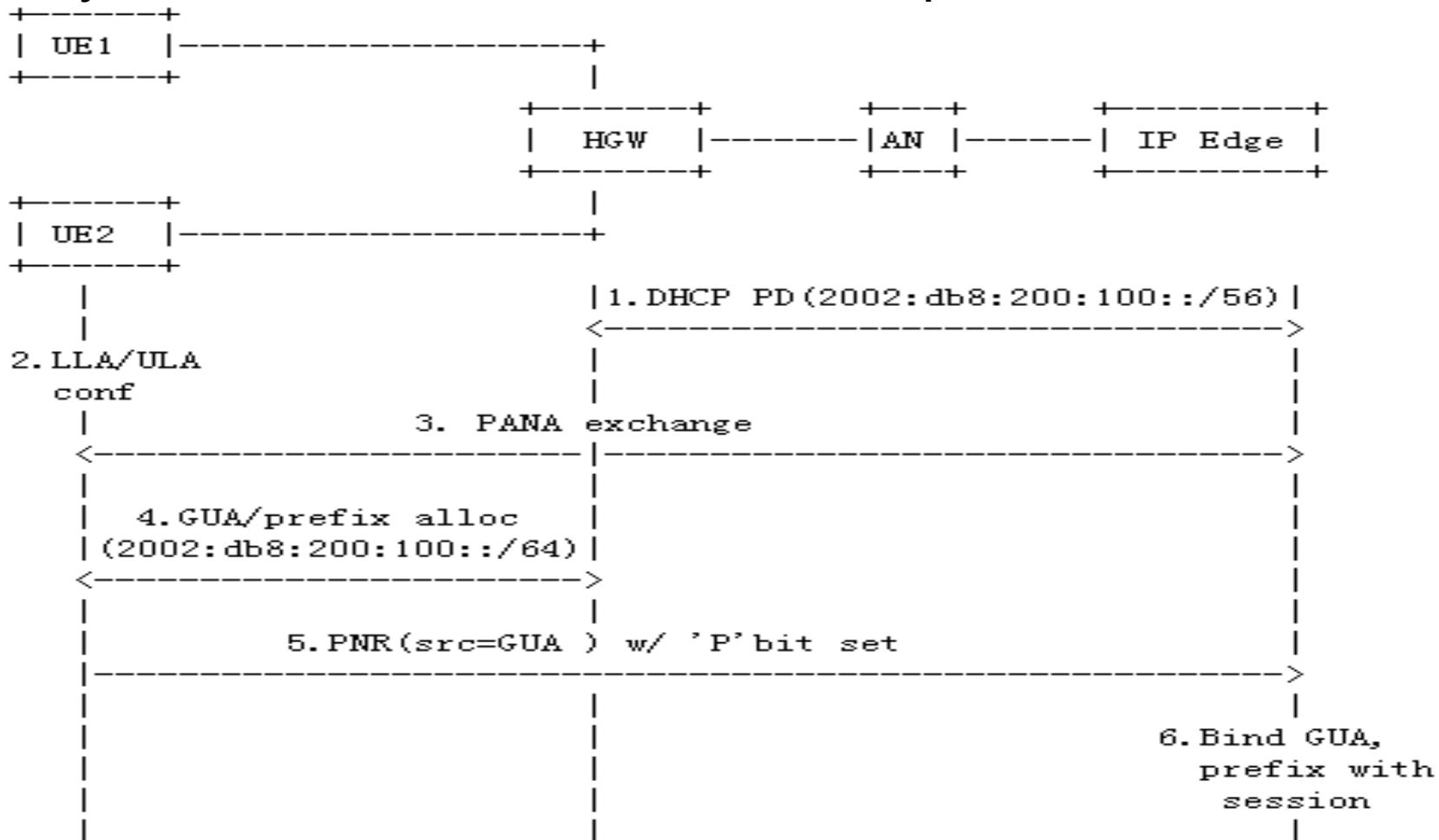
Figure 3: Message flow of IP/prefix reconfiguration in home network - 2
