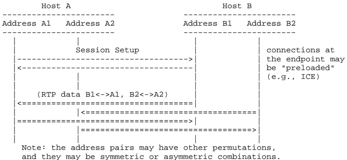
Figure 4: Bidirectional flow
