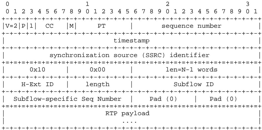
Figure 9: MP RTP header for subflow
