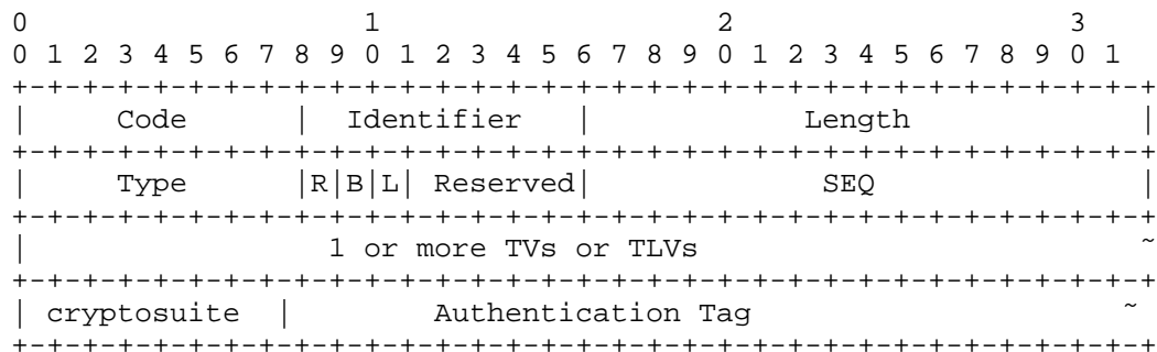
Figure 9: EAP-Initiate/Re-auth Packet
