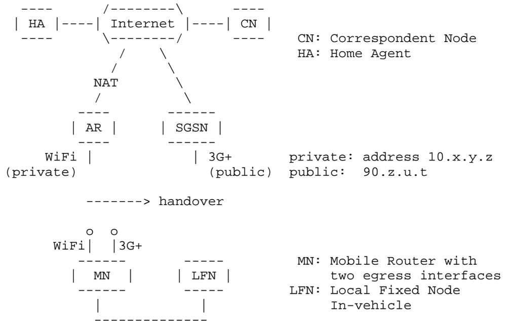
In this latter figure, the WiFi access offered by the Access Router is using a private address space. It uses DHCP to deliver IP Care-of Addresses which are non-routable in the Internet. On the other hand, the SGSN 3G+ wireless access offers IP addresses which are publicly routable in the Internet (public space).
