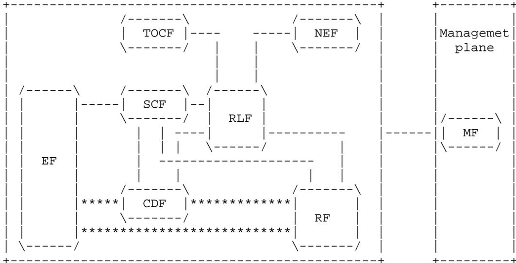
RLF in the above figure is equivalent to the peer of RELOAD. And NEF is equivalent to the Enrollment server of RELOAD. And MF is the function of network management. The specific descriptions of every function are as follows:
