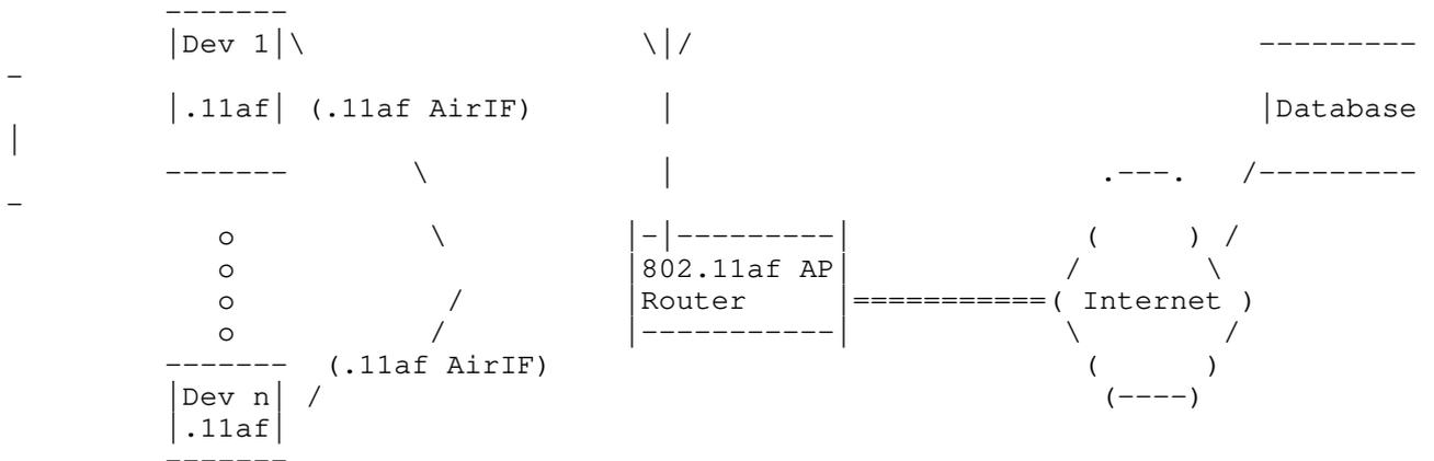
Figure 2: Hot-spot service using TV white space spectrum
