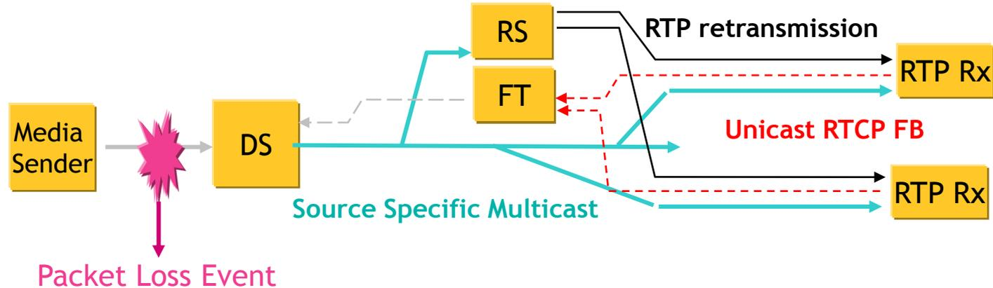
FB storm suppression realised by AVPF algorithm implemented by SSM RTP receivers
