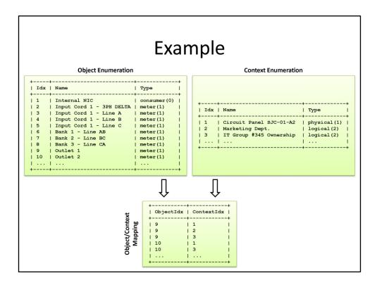
This is an example of how an entity can be mapped to a context. It is a simple table mapping, where membership in a context by an object is simple to derive for an NMS.
