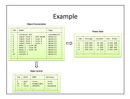
This is an example of how the various tables relate to one other. Here, we see a Power Distribution Unit described. The unit has a Three Phase input cord, which has child objects listed. (The relationship between parents and children is not shown due to space constraints.) Each object is given a unique index value, which is then used by sparse tables that extend the functionality in role-specific ways.
