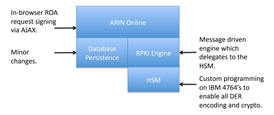
HSM coding is in C as extensions to IBM CCA. Libtasn1 used for DER coding.
