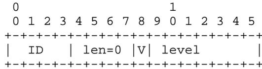
Sample audio level encoding using the one-byte header format
