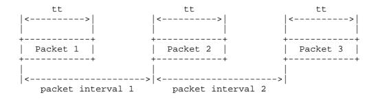
The packet interval between consecutive packets for each train sent by the Session-Sender and reflected by the Session-Reflector MUST be calculated and determined by the controller or an application or entity communicating with the controller. The packet interval MAY be constant within a train. Determination of the packet interval within a train as well as for consecutive trains for a given test session is implementation-specific.
