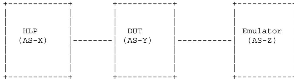
Figure 2 Three Node Setup for eBGP and iBGP Convergence
