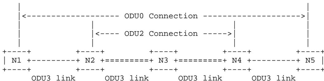
Figure 3 - Example of multiplexing hierarchy
