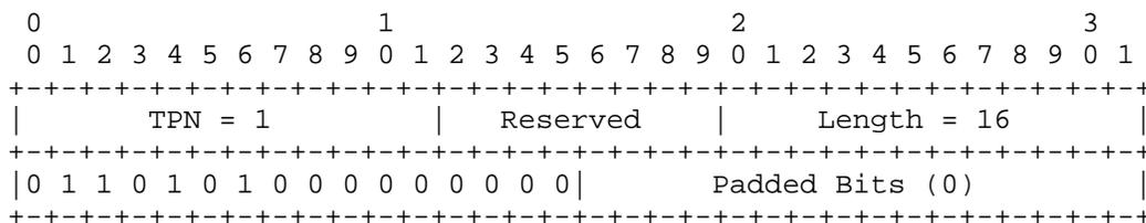
This above label indicates an ODU2 multiplexed into the 2nd, 3rd, 5th and 7th tributary slot of ODU3, wherein there are 16 TS in ODU3 (i.e., the type of the tributary slot is 2.5Gbps), and the TPN value is 1.
