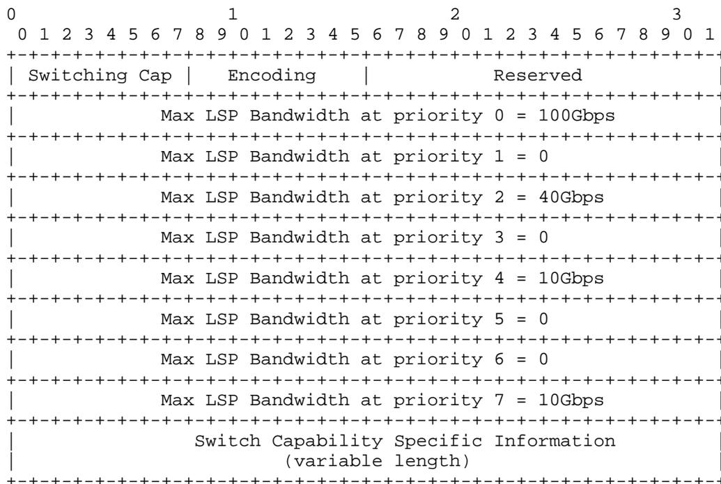
Figure 9: Example 1 - MAX LSP Bandwidth fields in the ISCD @T2
