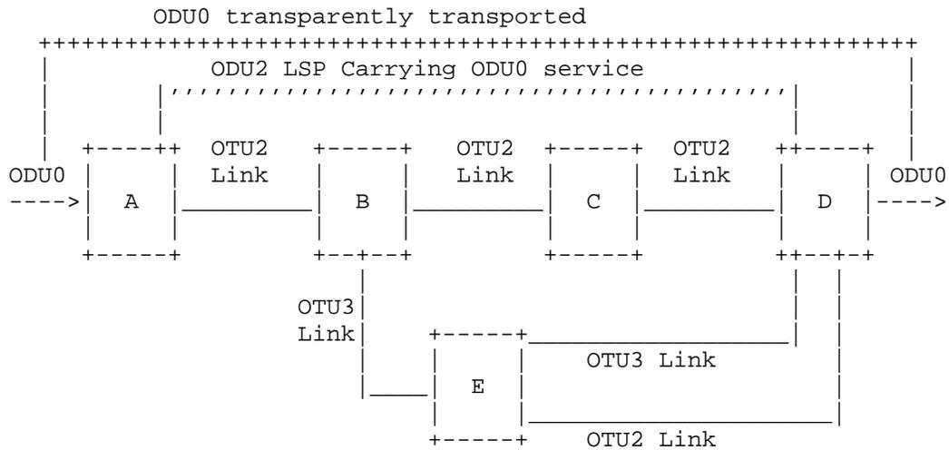
Figure 8: Switching and Terminating capabilities - Example 1
