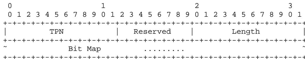
The ODU Generalized Label is used to indicate how the LO ODUj signal is multiplexed into the HO ODUk link. Note that the LO ODUj signal type is indicated by traffic parameters, while the type of HO ODUk link can be figured out locally according to the identifier of the selected interface carried in the IF\_ID RSVP\_HOP Object.
