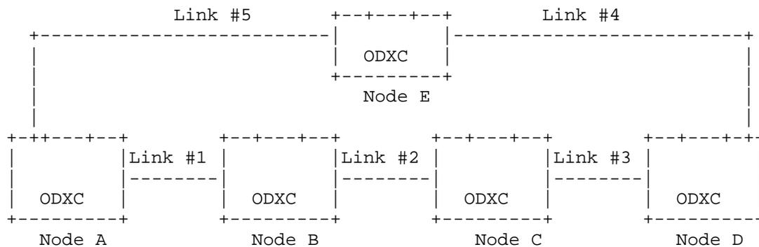
Figure 2 - Example Topology for LO ODU connection management
