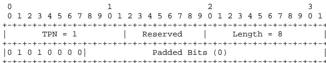
This above label indicates an ODU1 multiplexed into the 2nd and the 4th tributary slot of ODU2, wherein there are 8 TS in ODU2 (i.e., the type of the tributary slot is 1.25Gbps), and the TPN value is 1.
