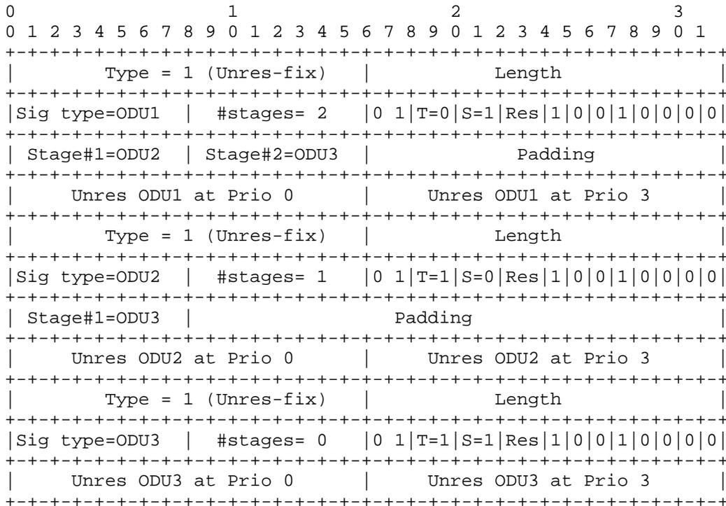
Figure 10: Example 2 - TSG, T and S utilization
