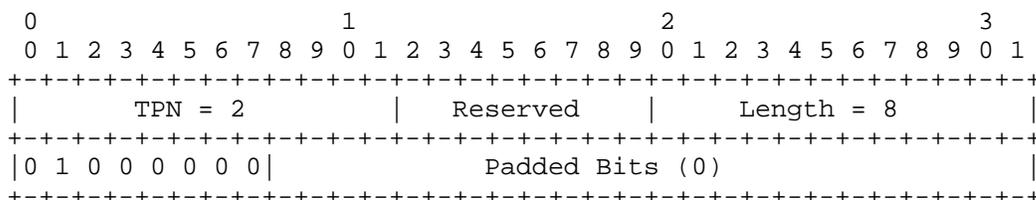
This above label indicates an ODU0 multiplexed into the second tributary slot of ODU2, wherein there are 8 TS in ODU2 (i.e., the type of the tributary slot is 1.25Gbps), and the TPN value is 2.
