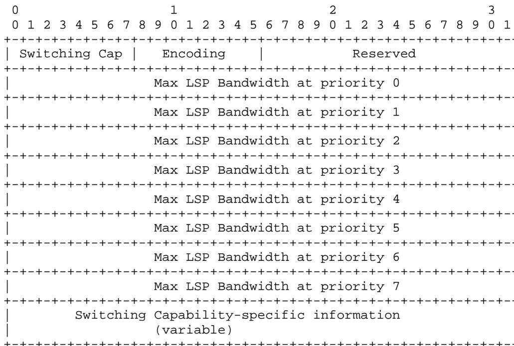
Maximum LSP BW is really not used for super channel connection. All the required information is in terms of spectral slices which are distributed within the ISCD specific portion of the ISCD for flex grid telink.
