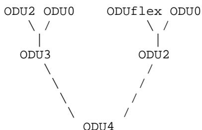
The ODU4 is the root of the muxing tree, ODU3 and ODU2 are containers directly multiplexed into the server and then ODU2, ODU0 are the leaves of the ODU3 branch, while ODUflex and ODU0 are the leaves of the ODU2 one. This means that on this traffic card it is possible to have the following multiplexing capabilities:
