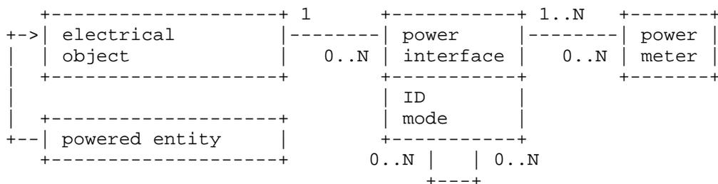
Figure 19: Basic Information Model of the PSU Layer
