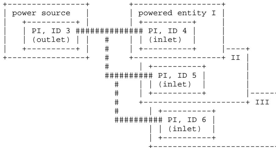
Figure 9: PSU Layer for a Single PS Supplying Multiple PEs.
