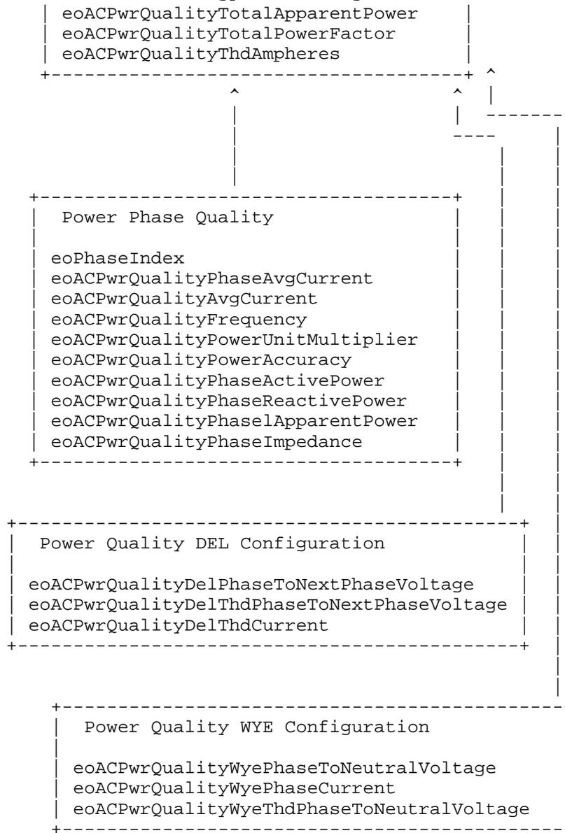
Figure 2: UML diagram for the powerQualityMIB
