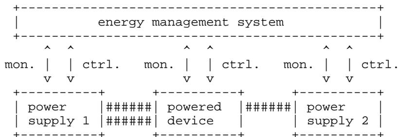
Figure 5: Multiple Power Supply for Single Powered Device
