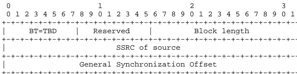
5.2. Definition of Fields in RTP Flow General Synchronization Offset Metrics Block
