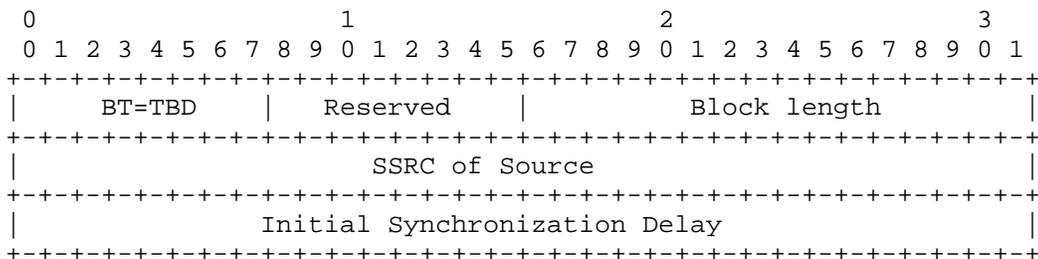
4.2. Definition of Fields in RTP Flow Initial Synchronization Delay Metrics Block
