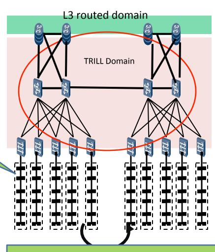
VMs can be moved to any rack without IP re-configuration on any switches
