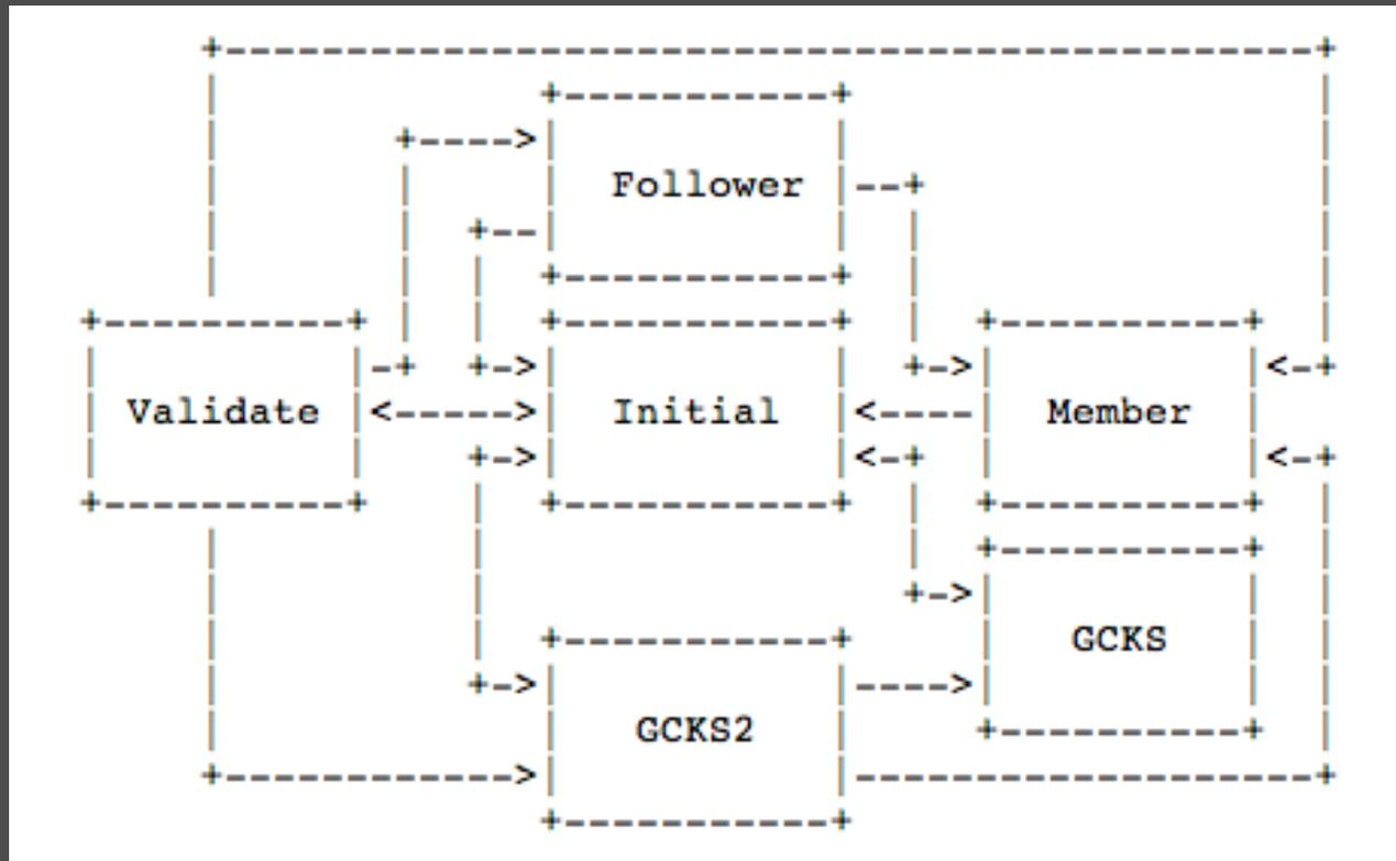
Router starts in Initial state and a router moves through the state machine to either member or GCKS depending on its priority.
