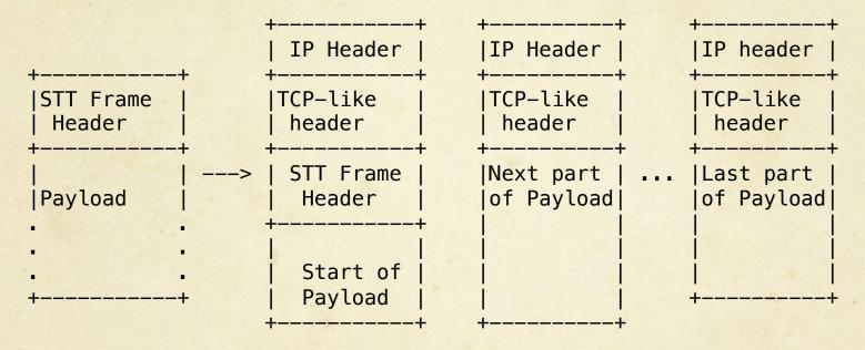
Original data frame is encapped with STT Header
