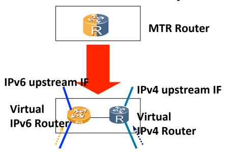
For simplification, we use two virtual Routers to replace MTR Router
