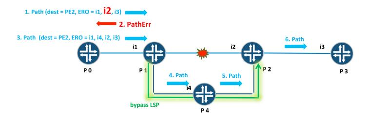
What will happen, if there is a link/node failure along the path when the initial Path message is being signaled?
