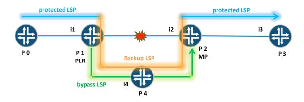
The LSP appears as if it was originally set up along the desired path and failed over to the bypass LSP.
