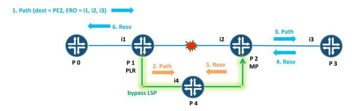
PLR (point of local repair) reroutes LSP through an existing bypass LSP.
