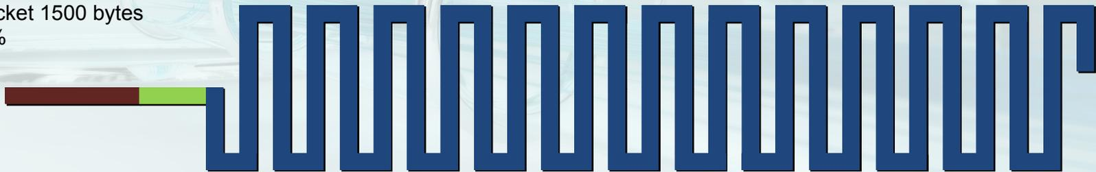
One IPv6/UDP/RTP packet of VoIP with two samples of 10 bytes
