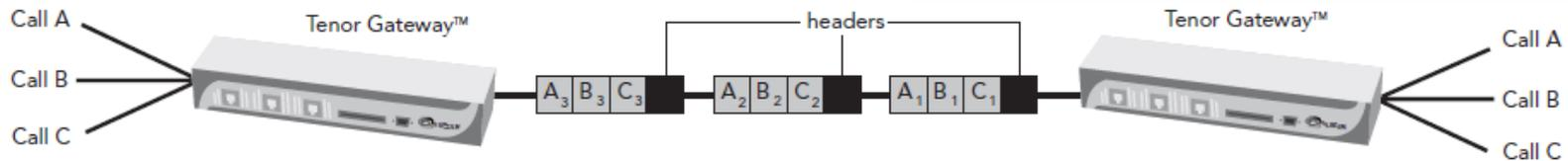
Quintum's *PacketSaver* technology multiplexes small voice/fax-over-IP packets into larger packets to increase network efficiency, thereby reducing the total amount of packet "overhead" required to transmit voice and fax over IP networks
